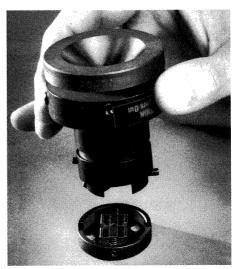
Reassemble Springs to Guides and install in Receptacle Housing.
