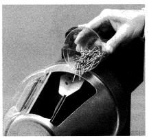
2. Open the reservoir cover and load approximately 1000 POP Rivets into the hopper.
