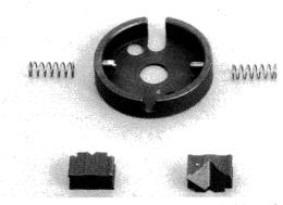
Clean Guides and Springs in a suitable solvent: Dry parts thoroughly. *DO NOT* lubricate Guides as this allows dirt to accumulate and cause sticking and sluggish operation.
