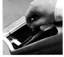
3. Manually place 6-8 rivets into the feed track.
