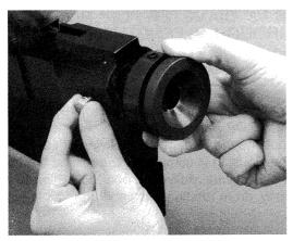
Remove Receptacle Housing Assembly by loosening the side mounted thumb screw.
