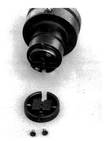
Remove rear cover of Receptacle Housing and remove the two Rivet Guides and Springs from inside Housing, noting Guide orientation. Clean Housing Slot.
