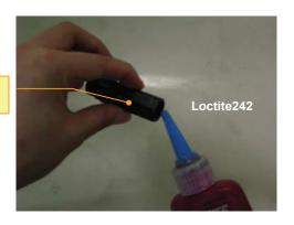
Screw Pulling Head Ass'y to Hydraulic Piston Ass'y
