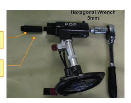
Apply Loctite242 on the thread part of Pulling Head Ass'y.
