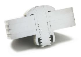
Lock groove on pin engages shoulder on rivet head, while the support ring "double locks" the pin within the bulb.
