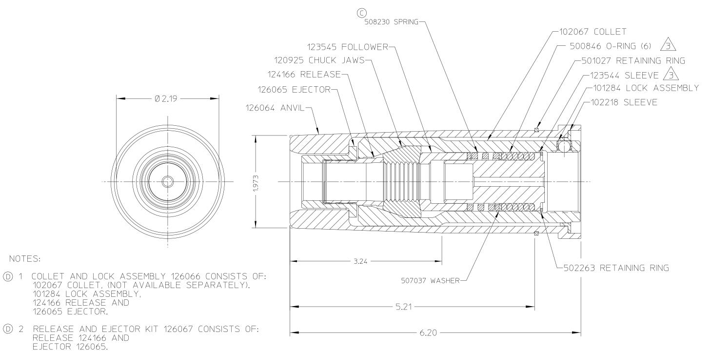
ASSEMBLE SLEEVE AND O-RINGS PER HUCK SPEC. 42-491.
