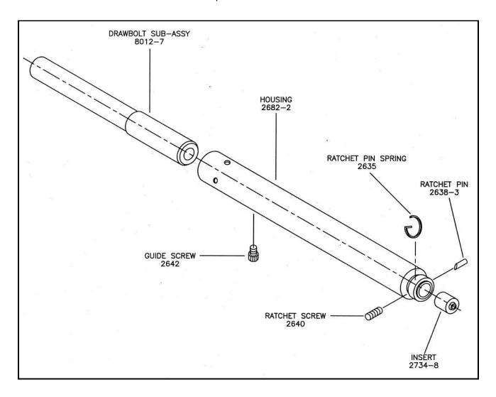
8012-7 Drawbolt Sub Assembly Exploded View
